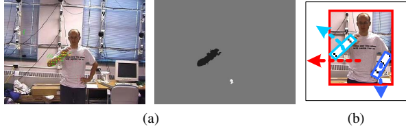
Fig.8. (a) At each frame, only some parts of the body (those in motion) can be segmented. (b) In the body area, several different motions may exist simultaneously.
