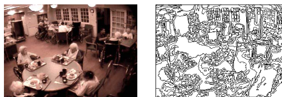
Fig. 5. Region over-segmentation based on color.
