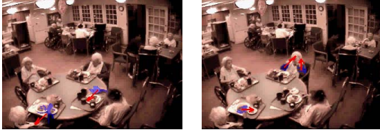
Fig.11. Articulated motion segmentation in a dining room video. Blue masks indicate segmented moving regions, and red arrows are estimated motion vectors for each region.
